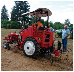
rear-mounted tractors. Participants were able to try the new Tilmor cultivating tractor, and test out hand-steering rearmounted toolbar setups.
