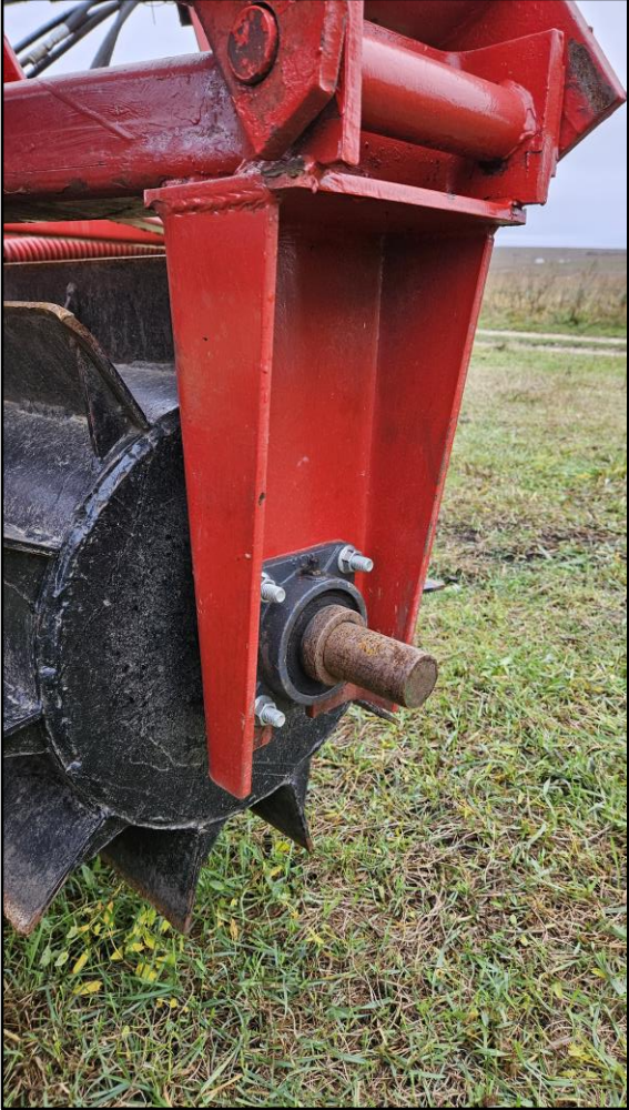
Assembled hanging bracket attached to finished crimper drum using bearing.
