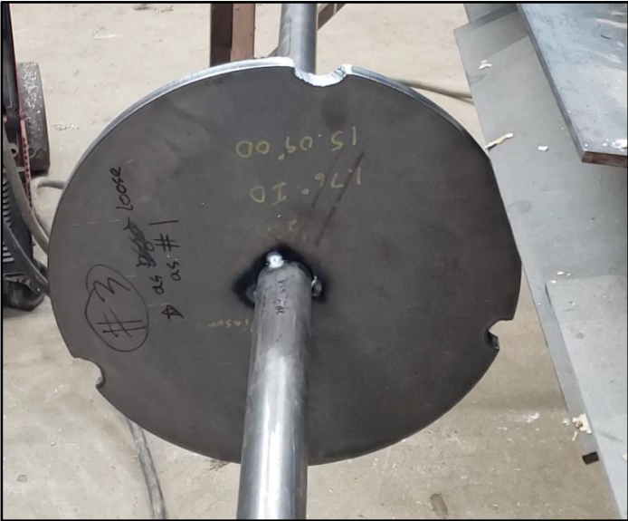
Three notches were cut into the center support plate to allow water to flow freely throughout the center drum.
