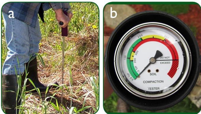
**FIGURE 3 a and b.** Measuring surface and subsurface hardness with a penetrometer. Source (b): [agriculturesolutions.com](http://agriculturesolutions.com)
