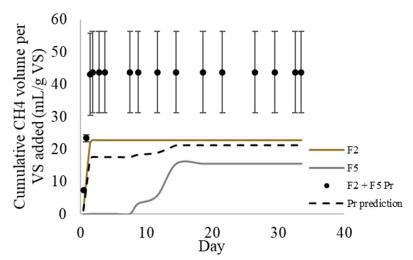
Figure 11: Co-digestion results for starch (F2) and soap stock (F5). F2 + F5 Eq = 1:1 ratio of VS; F2 + F5 Pr = ratio of VS is proportional to what full-scale digester receives. Points indicate treatment averages with error bars showing standard deviation. Dashed lines indicate treatment prediction assuming no synergy.
