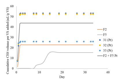
Figure 10: Cumulative specific methane production for starch (F2) and soap stock (F5). F2 + F5Pr = ratio of VS is proportional to what full-scale digester receives.
