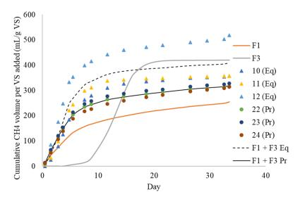
Figure 4: Cumulative specific methane production for manure (F1) and slaughterhouse waste (F3). F1 + F3 Eq = 1:1 ratio of VS; F1 + F3 Pr = ratio of VS is proportional to what full-scale digester receives.
