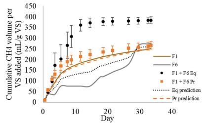
Figure 9: Co-digestion results for manure (F1) and filter press slurry (F6). F1 + F6 Eq = 1:1 ratio of VS; F1 + F6 Pr = ratio of VS is proportional to what full-scale digester receives. Points indicate treatment averages with error bars showing standard deviation. Dashed lines indicate treatment prediction assuming no synergy.
