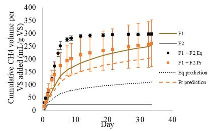
Figure 3: Co-digestion results for manure (F1) and starch (F2). F1 + F2 Eq = 1:1 ratio of VS; F1 + F2 Pr = ratio of VS is proportional to what full-scale digester receives. Points indicate treatment averages with error bars showing standard deviation. Dashed lines indicate treatment prediction assuming no synergy.
