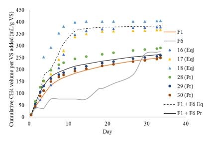
Figure 8: Cumulative specific methane production for manure (F1) and filter press slurry (F6). F1 + F6 Eq = 1:1 ratio of VS; F1 + F6 Pr = ratio of VS is proportional to what full-scale digester receives.
