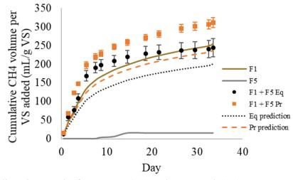
Figure 7: Co-digestion results for manure (F1) and soap stock (F5). F1 + F5 Eq = 1:1 ratio of VS; F1 + F5 Pr = ratio of VS is proportional to what full-scale digester receives. Points indicate treatment averages with error bars showing standard deviation. Dashed lines indicate treatment prediction assuming no synergy.
