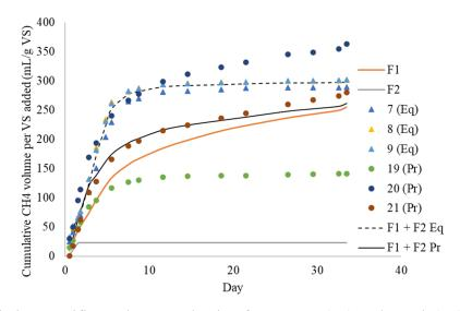
Figure 2: Cumulative specific methane production for manure (F1) and starch (F2). F1 + F2 Eq = 1:1 ratio of VS; F1 + F2 Pr = ratio of VS is proportional to what full-scale digester receives. Points indicate individual digesters (7-9 are Eq treatment, 19-21 are Pr treatment).
