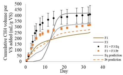
Figure 5: Co-digestion results for manure (F1) and slaughterhouse waste (F3). F1 + F3 Eq = 1:1 ratio of VS; F1 + F3 Pr = ratio of VS is proportional to what full-scale digester receives. Points indicate treatment averages with error bars showing standard deviation. Dashed lines indicate treatment prediction assuming no synergy.
