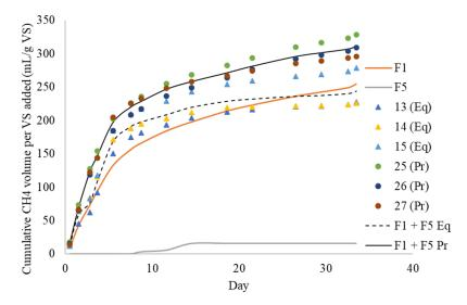
Figure 6: Cumulative specific methane production for manure (F1) and soap stock (F5). F1 + F5 Eq = 1:1 ratio of VS; F1 + F5 Pr = ratio of VS is proportional to what full-scale digester receives.
