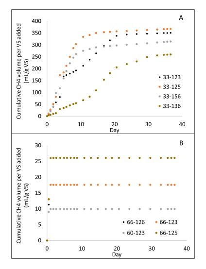
Figure 7: Cumulative methane production curves for the low (A) carbohydrate and high (B) carbohydrate treatments.
