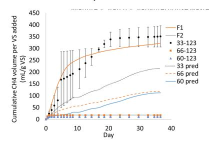
Figure 2: Cumulative methane production curves for the three manure, starch, and slaughterhouse waste (F1+F2+F3) treatments. Error bars indicate standard deviation and points represent treatment averages. Dotted lines indicate prediction curves based on weighted average of mono-digestion controls.
