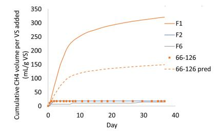
Figure 6: Cumulative methane production curve for the manure, starch, and filter press slurry (F1+F2+F6) treatment. Error bars indicate standard deviation and points represent treatment averages. Dotted line indicates prediction curve based on weighted average of mono-digestion controls.
