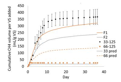
Figure 3: Cumulative methane production curves for the two manure, starch, and soap stock (F1+F2+F5) treatments. Error bars indicate standard deviation and points represent treatment averages. Dotted lines indicate prediction curves based on weighted average of mono-digestion controls.
