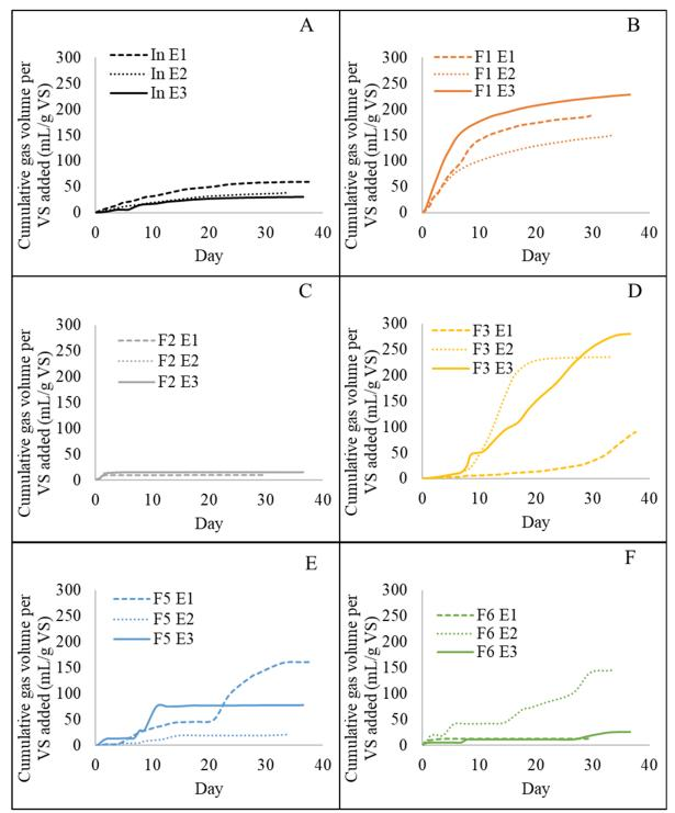
Figure 1: Comparison of mono-digestion results between E1, E2, and E3.
