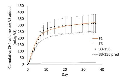
Figure 5: Cumulative methane production curve for the manure, soap stock, and filter press slurry (F1+F5+F6) treatment. Error bars indicate standard deviation and points represent treatment averages. Dotted line indicates prediction curve based on weighted average of monodigestion controls.
