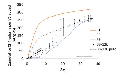
Figure 4: Cumulative methane production curves for the manure, slaughterhouse waste, and filter press slurry (F1+F3+F6) treatment. Error bars indicate standard deviation and points represent treatment averages. Dotted lines indicate prediction curves based on weighted average of mono-digestion controls.
