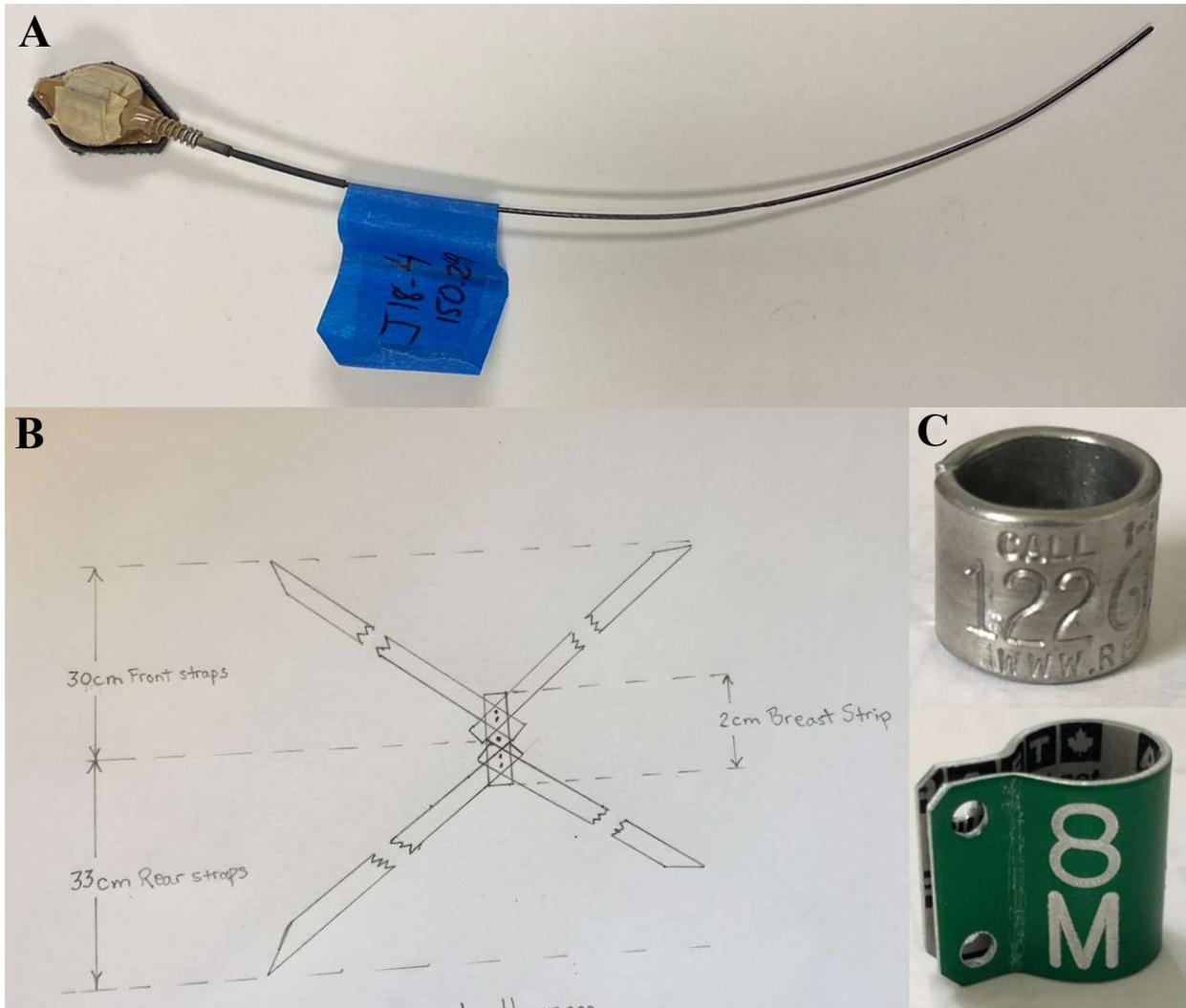
**Figure 3.2.** (A) American Wildlife Enterprises backpack AWE-Q VHF transmitter; (B) backpack-style harness design tailored to pueo (B. Milsap, J. Pagel, United States Fish and Wildlife Service; J. Penniman, Maui Nui Seabird Recovery Project, personal communication); and (C) aluminum federal and visual identification bands used to tag and band pueo in 2019 on the island of O‘ahu, Hawai‘i, USA.
