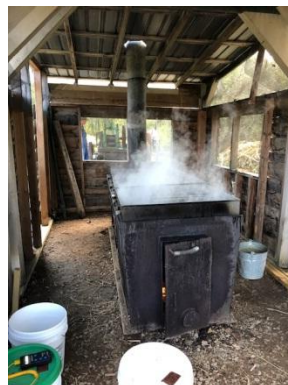
The cook-down process begins on the evaporator. Roughly 7 gallons of juice produce a gallon of syrup.
