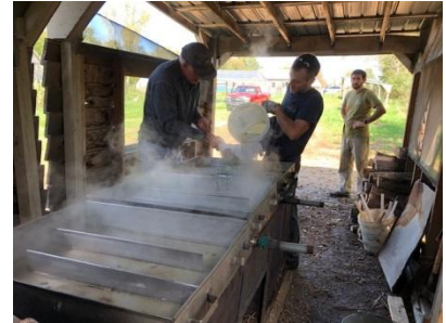
Sorghum juice is boiled down and strained atop a wood-fired evaporator to create a thickened, golden liquid before final finishing.
