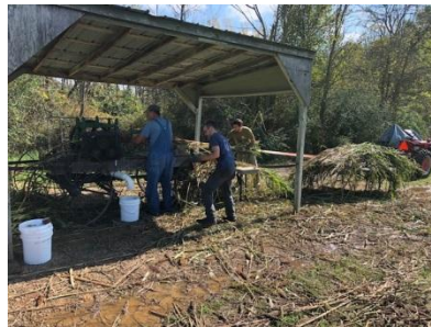
The stalks are hand delivered through a 120-year-old press to begin the process. Pressed canes are fed to local animals, making it a zero-waste operation.
