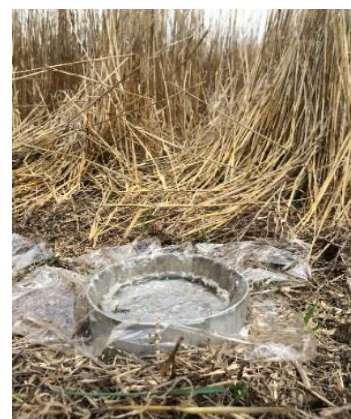
Figure 2. Soil water infiltration test conducted following wheat harvest.
