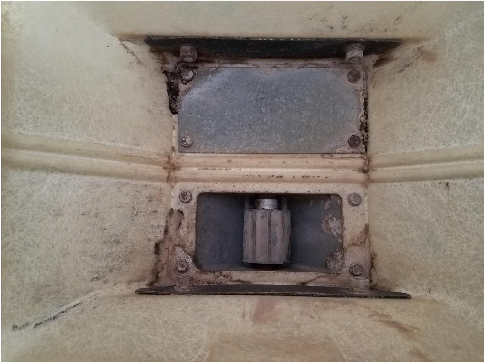
Figure 1. Planter insecticide box and metering unit used to band-apply gypsum.
