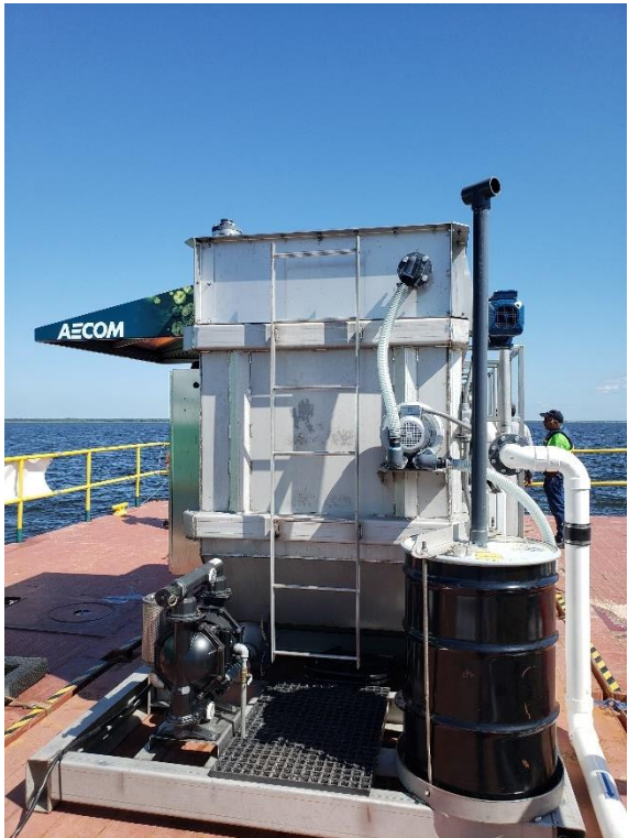
Figure 1. Mobile, custom-built algae harvester unit of AECOM. The harvester was working at lake Jesup in Central Florida. Pictures also showing the working principle of the unit
