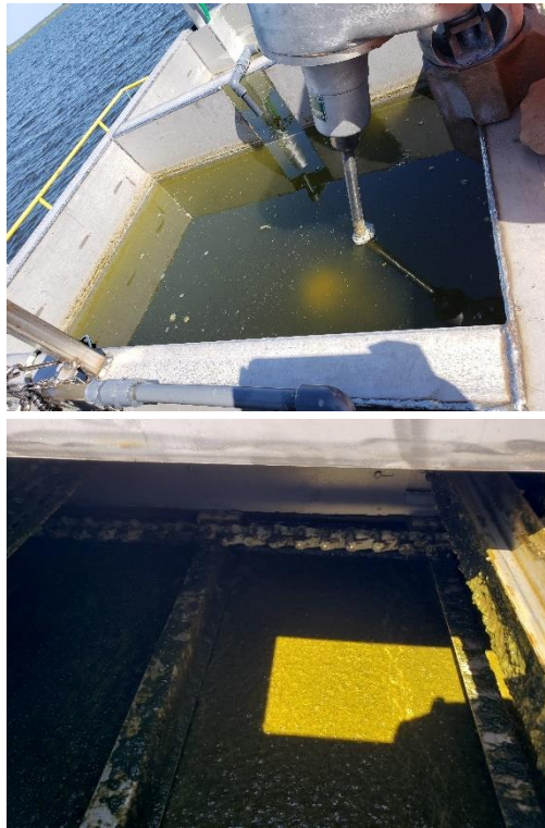
Figure 1. Mobile, custom-built algae harvester unit of AECOM. The harvester was working at lake Jesup in Central Florida. Pictures also showing the working principle of the unit
