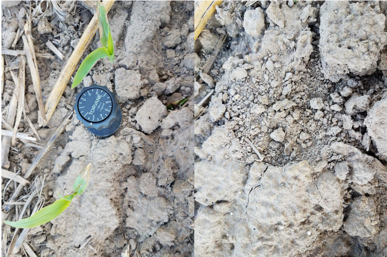
Figure 3. Measuring crust strength with a Torvane shear penetrometer, 30DAE. Photo on the right indicates the degree of crusting which developed after emergence.
