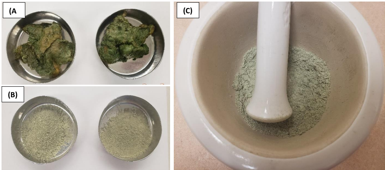
Figure 5A. Pictures of (A) small sample of collected wet cyanobacterial mat (B) dried and ground cyanobacteria and (C) process of grinding in mortar and pestle. Commercial grinding machine (Model # BL-230) will be used to process the biofertilizer required for greenhouse study and field trials.
