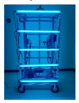
Fig. 1. UV-C cart assembled for this project with parts procured from multiple suppliers.
