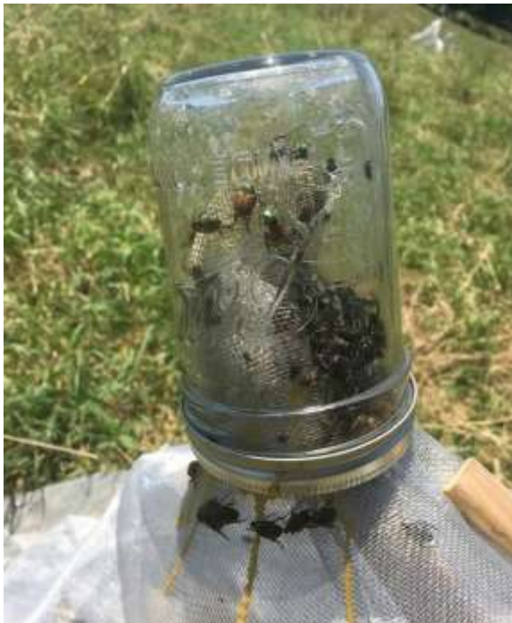
Figure 5: Emerging flies climb into the jar at top of trap and are retained.
