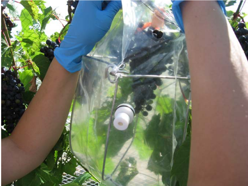
Marquette cluster in polyvinyl film (Tedlar) enclosure with stainless steel cage and solid phase microextraction (SPME) port. Photo by Somchai Rice.
