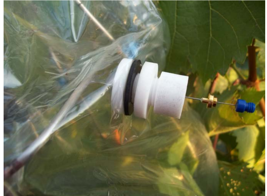
Teflon SPME port with teflon backed septum. PDMS/DVB SPME extraction, exposed fiber, 30 minutes at ambient temperature. Photo by Somchai Rice.
