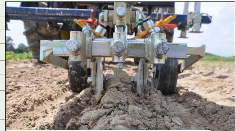
**Figure 3:** Duo hilling discs set to throw soil into the crop row. Looking towards the direction of travel
