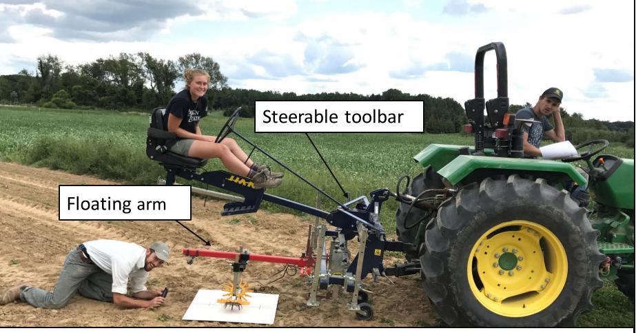
Figure 3: Tractor, steerable toolbar, floating arm, finger weeders
