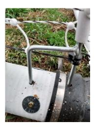
9- Clip the top strand of the fence to the top cap of the fiberglass post.
