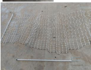
Measure and mark each spike at 3.5" from the horizontal step of the spikes. While wearing safety glasses, use a metal chop saw or an angle grinder to cut the spikes at that mark. Remember to do this to the terminal posts that are still connected to the netting, too.
