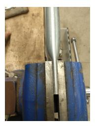
Use a 3/8" drill bit to drill a hole through the center of the flattened ends of the pipes. The lag screw should be able to fit through the hole.
