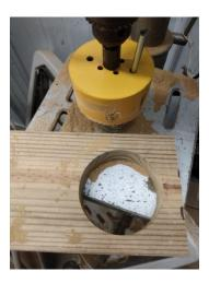
With all the lumber cut to length and the holes cut in place, you're ready to take the materials to the coop and assemble the mount.
