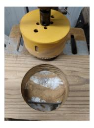
Cut another 3-3/4" hole in the vertical piece. Put the center of the hole at exactly 2.75" from the end of the lumber.
