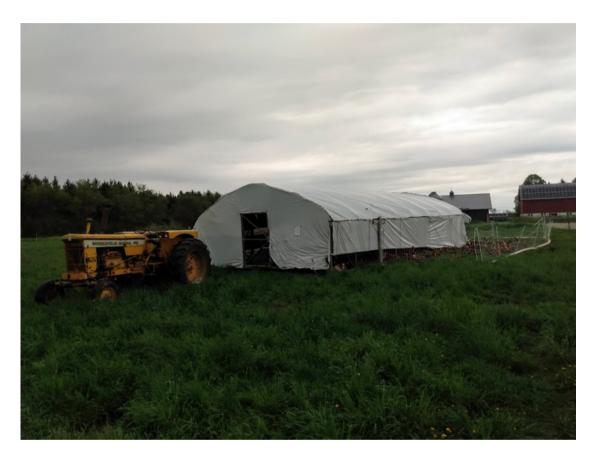
It's important to keep in mind that this adds a bit of drag to the coop, which requires more power to pull. I bought a heavy 75 hp tractor dedicated to moving coops. With a lightweight 30 hp tractor, I was ripping up the pasture trying to move these coops.
