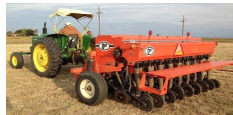
Interseeding alfalfa into native grasses using a Tye no-till drill in October 2015.
