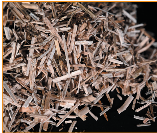
Figure 11. (top): Retted bast fiber. Figure 12. (middle): Retted secondary bast fiber, or tow fiber. Figure 13. (bottom): Hurd fiber.
