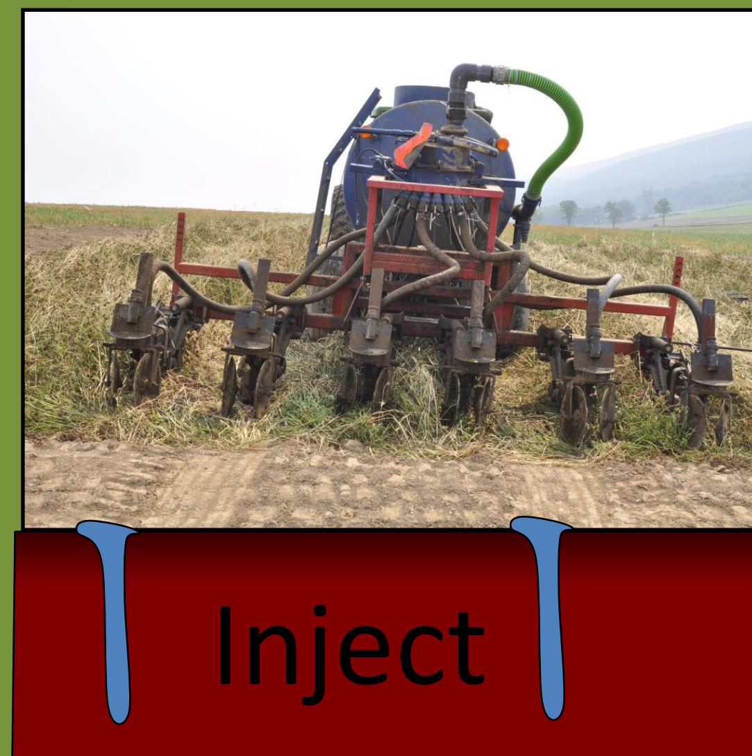
Figure 3. Manure injection method
