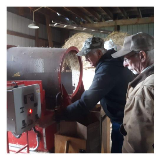
Leonard Reggie, left, and Rodney Leighow go over the startup procedure for a switchgrass chopper. The machine was built with funds from a USDA grant and chops switchgrass into a material that can be used for poultry bedding and garden mulch. Tom Venesky
