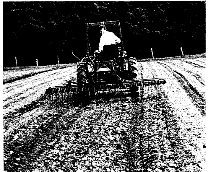
Mark Miller has demonstrated excellent weed control in strawberries with a Lely Springtine(see entry 44).
