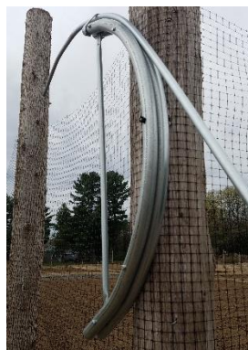
Bending EMT posts into hoops with the Hoop Bender
