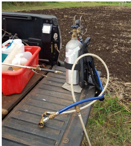
CO 2 sprayer set up
