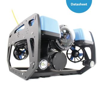
waters, with a standard 100m depth rating and up to 300m tether lengths available.
