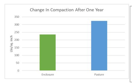
This graph shows the average soil compaction readings for the season of the enclosure and the pasture. The readings were taken with in a 20-foot radius of each other. The enclosure readings show that there is a 28% reduction in compaction after one year.
