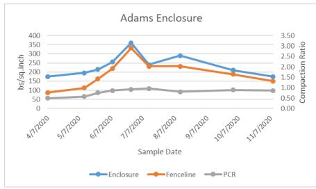
This graph shows the compaction within the exclusion enclosure compared to the fenceline. Notice that the red and blue compaction lines get closer during the early season. This indicates that the enclosure soil is getting closer to the "optimum" compaction of the fenceline.
