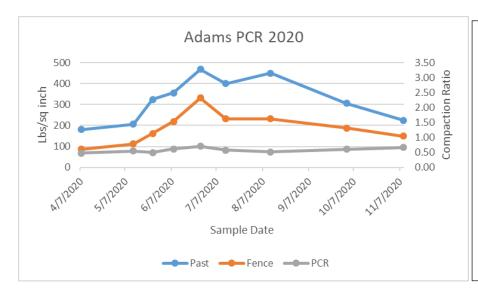
As expected, the compaction in the paddock was higher than the fenceline. Both area's compaction increased as the soil dried out. The grey line is connected to the right hand Y axis. It showed that as the compaction increased the ratio stayed relatively constant. This was a major goal of this project.
