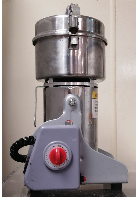
Figure 4. A grain grinder for milling the papaya seeds into PGS.
