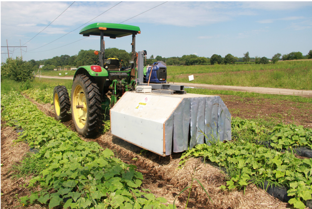
Completed UV treatment unit shown in a row of the trial plot at Ward's Berry Farm in August, 2020.
