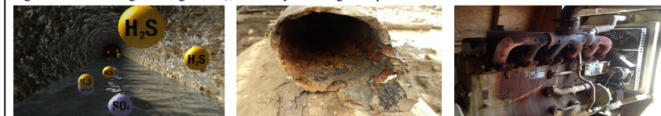
Figure 1. H<sub>2</sub>S production from sulfate rich wastewater (left) and effects of H<sub>2</sub>S induced corrosion in pipelines and generators (middle, right).
