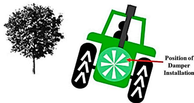
**Figure 7.** Position of damper installation for precision sprayer airflow control.
