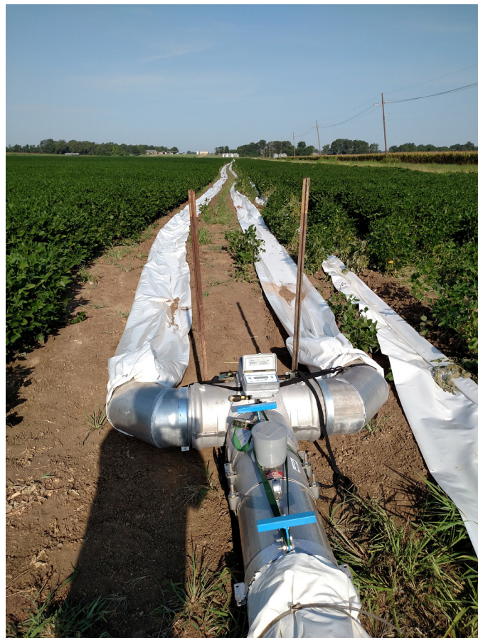
Surge valve in a soybean field. (Courtesy of Bruce Garner, ANR agent West Carroll parish.)
