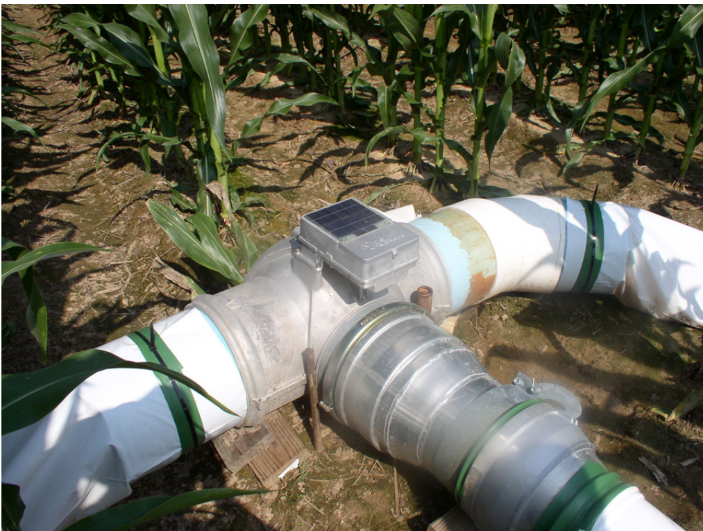
Photo 2. Surge valve in a corn field. (Courtesy of Bruce Garner, ANR agent West Carroll parish.)
