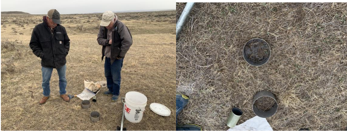
In the field, Rick Caquelin and Peter Donovan setting up infiltration rings
