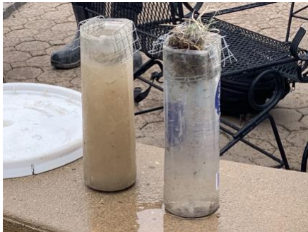
Slake test: low organic matter and poor structure versus higher organic matter and strong granular structure (aggregation)
