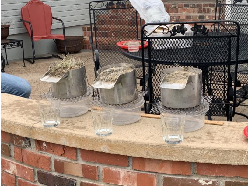
Infiltration Demo: Three soil samples taken in close proximity, but with different vegetation cover and soil properties
