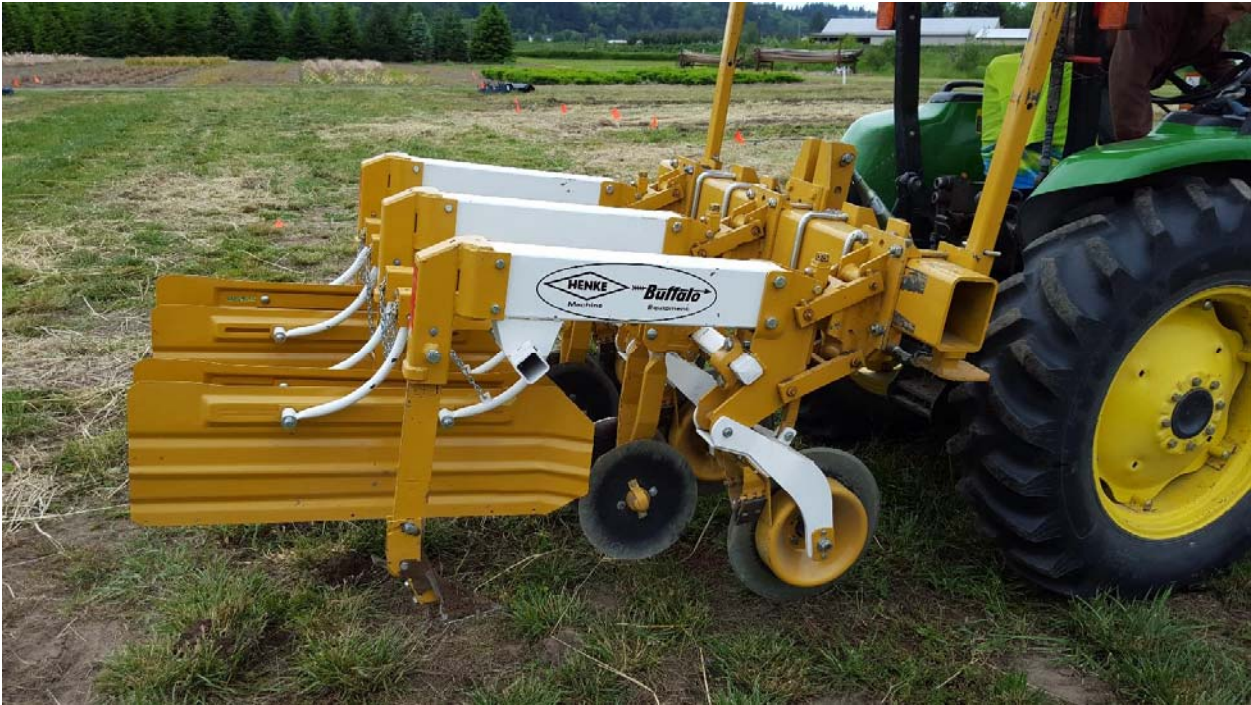
Henke Buffalo 6600 Cultivator, 2 row on 75" 5X7 Bar. Open top shields.
