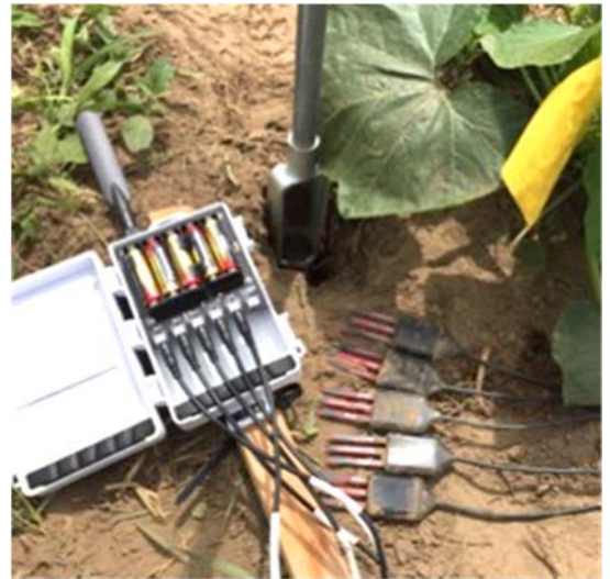
Figure 13. Decagon EM50G Logger with 5TE volumetric and temperature sensors.
