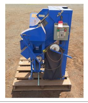
Agriculex Corn Sheller with Rubber Rollers will produce clean, whole kernels for seed and food products and will make shelling cobs go faster than hand shelling.
