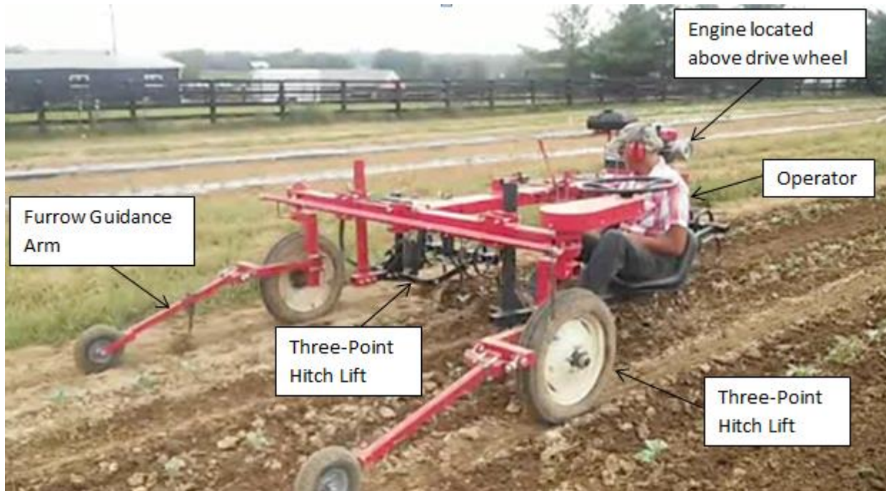
Figure 1. New prototype of the three wheeled machine with furrow guidance.
