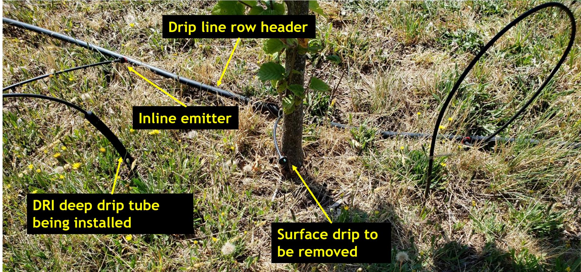
This is the typical arrangement for the DRI deep drip units. Arranged on both sides of the tree and about the width of the current canopy.
