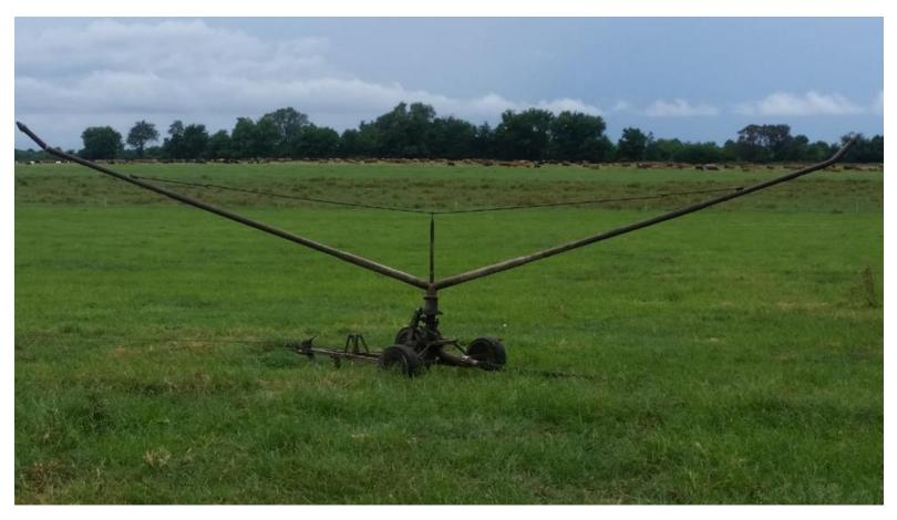
Figure 9: Low-pressure traveling gun (Spider). Irrigator is pulled across the paddock via a cable and ratchet powered by water pressure turning the arms. The water line is puled behind the irrigator. This can limit the type of forage species irrigated due to the water line
