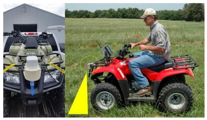
Figure 1: Front-mounted Senix sensor system implemented on ATV for measuring pasture height. Sound waves from the sensor reflect off the forage. The time difference between the tare value (zero) and forage indicate forage height in mm.
