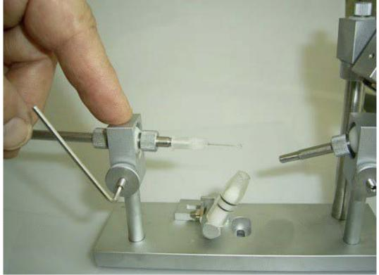
Height Adjustment of the Queen Holder Tube, Model 102
