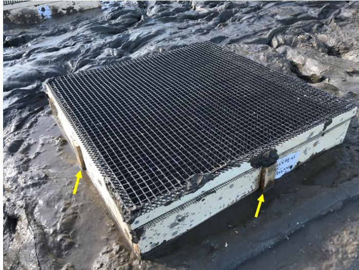
Figure 6. A 2-ft x 2-ft wooden box. Yellow arrows point to wooden strapping stakes (24-inches long) that are pushed into the soft sediments to the height of the box bottom. Two screws through the top of the strapping into the side of the box secure the box in place. Four stakes were used for the large boxes, and two for the small boxes.
