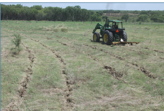
A tractor pulling the subsoil plow equipped with two 29-inch shanks.
