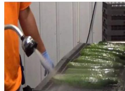
Using a sprayer head and sufficient water pressure is important for removing the soil as well as not bruising or harming the product's delicate skin.
