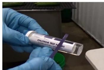
Choosing the correct sanitizer, and pH of your wash water is critical. pH, Chlorine and Peroxyacetic Acid concentration can be measured by testing strips.
