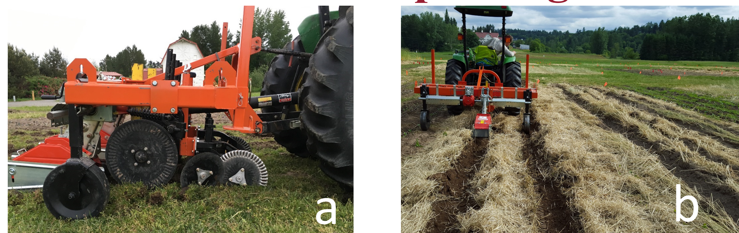
Figure 2. Custom-built powered strip tiller side view (a) and working in heavy flail-mowed rye residue (b)
