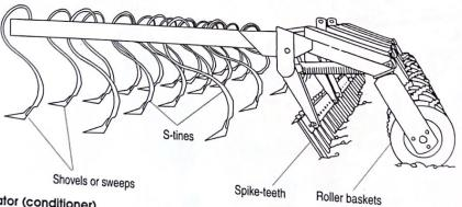
Figure 9.8 Field cultivator (conditioner) Source (a.): Adapted from Unverferth Manufacturing Co., Inc. mercial bed-former. Press pan units gather soil and form it into a firm bed. Some bed-forming units can also apply fertilizer and lay plastic mulch, and/or drip tape.
