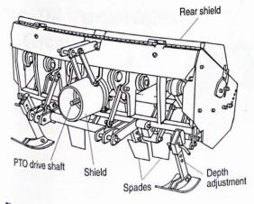
Figure 9.5 Spading machine Source: Adapted from Celli, S.p.A, Italy
