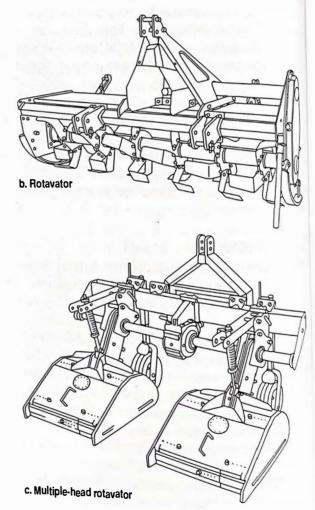
Figure 9.4 Rototiller, rotavator, and multiple-head multivator
