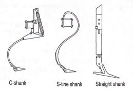
Shanks have a tool (such as a shovel or sweep) attached at the bottom. In general, C-shanks vibrate slightly; S-tine shanks vibrate vigorously; and straight shanks are rigid.
