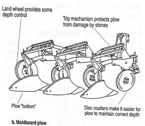
Figure 9.1 Moldboard plow with three bottoms Source (a.): Adapted from Brillion Iron Works, Inc.
