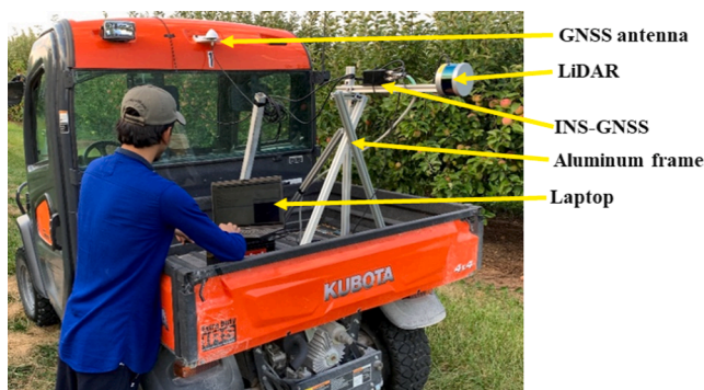
Fig. 4. Integrated hardware system for canopy position corrections.
