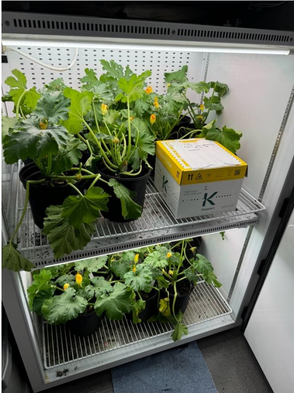
Growth Chamber (Percival) used to implement different temperature treatments on the plants and bumblebee micro colonies (Koppert USA).
