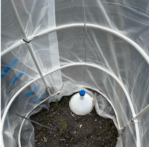
Open-Top-Chamber prototype with weather station inside.
