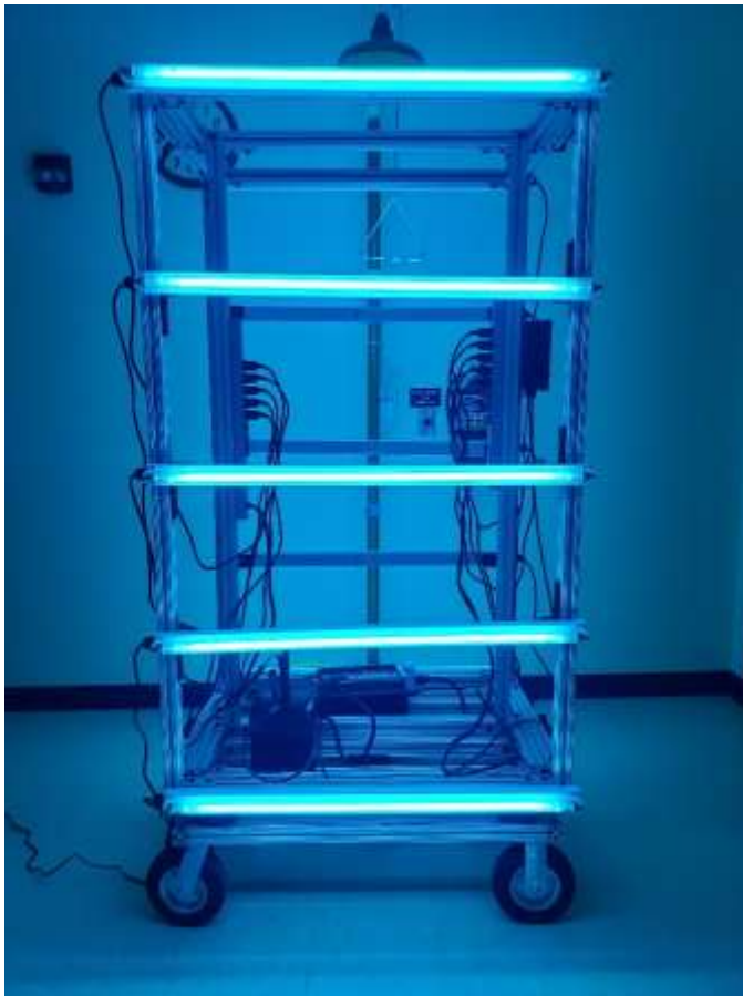
Fig. 1. A custom-built UV-C cart that can be driven in between tomato rows at a designated speed to get powdery mildew infected tomato plants exposed to UV-C for a pre-optimized time.
