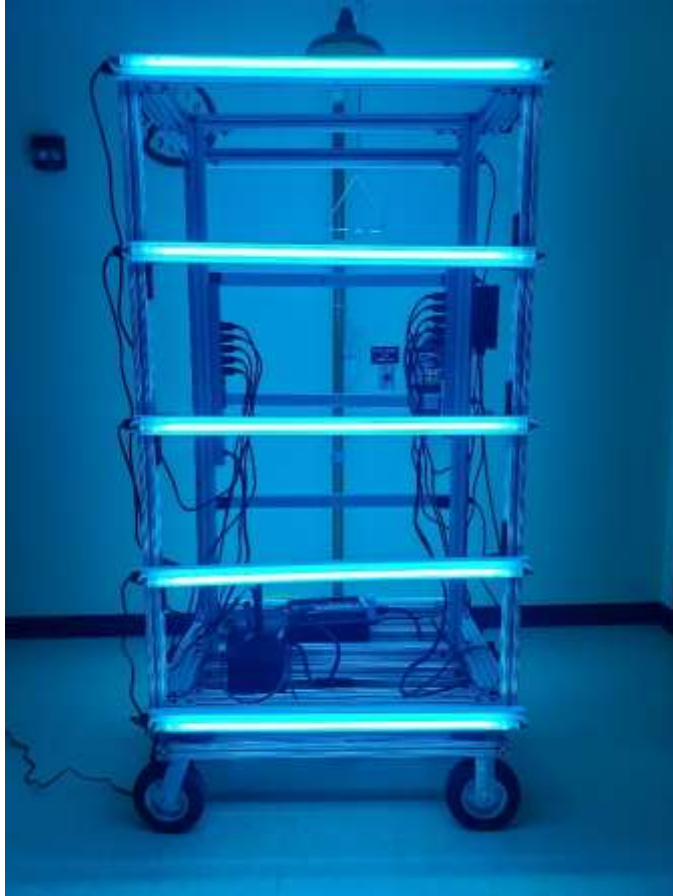
Fig. 1. A custom-built UV -C cart that can be driven in between tomato rows at a designated speed to have powdery mildew infected tomato plants exposed to UV-C for a pre-optimized time.
