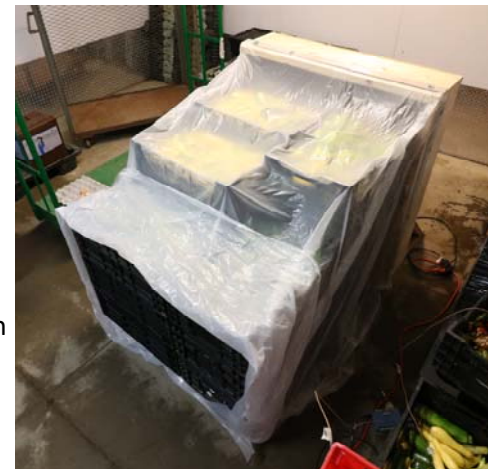
▲ This Pallet sized Forced Air Cooler was easily constructed in an afternoon with decking screws, dimensional lumber and plastic sheeting.
