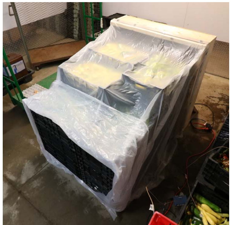
▲ This is a 4 foot tall version of a simple, portable forced air cooler. It is being used to cool a mixed pallet of fresh picked zucchini, summer squash, and peppers.
