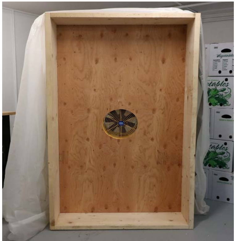
▲ This Pallet sized Forced Air Cooler was easily constructed in an afternoon with decking screws, dimensional lumber and plastic sheeting.
