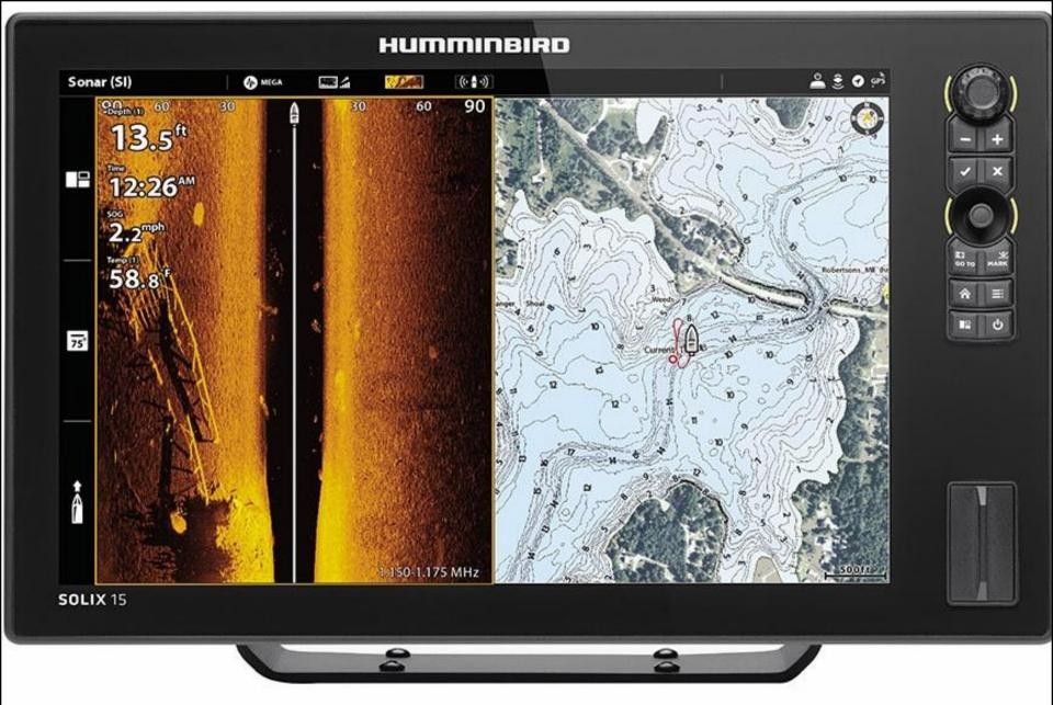
Example of a sidescan image (left side) and navigational aid (right side) in a split plot display on a Humminbird Solix 15 Fish Finder
