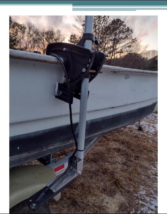
The fiberglass reinforced electric trolling motor mount with transducer mounted pole clamped to the bow of our 19' Carolina Skiff
